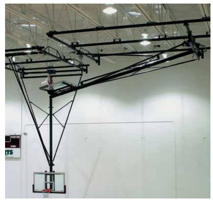
Most popular backstop, the TF-20 Basketball Backstop features a front-braced, ceiling-suspended, forward-folding backstop. Backstops are custom designed so the lateral sway brace intersects the main mast at approximately 54" (1.37 m) above the goal and 18" (46 cm) above the backboard; to ensure maximum rigidity.
